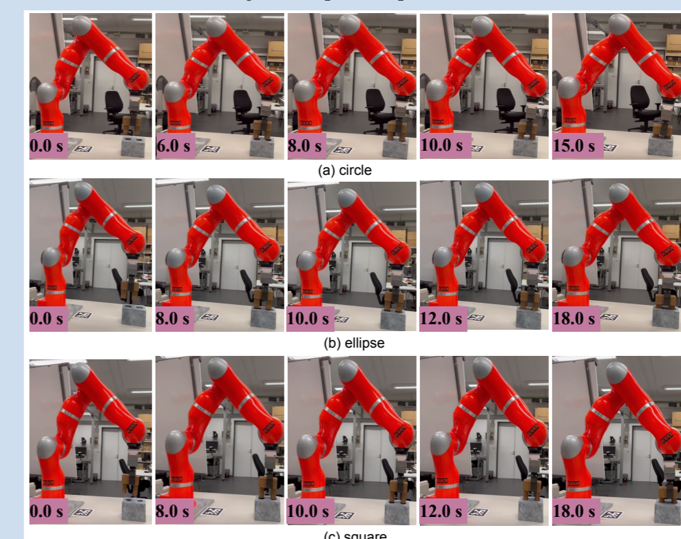
Figure 5: Example of the proposed solution on multiple peg-in-hole assembly for different trained object shapes (a) circle (b) ellipse (c) square.
