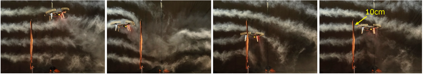
Fig. 2: Agile flight through narrow gates. Neural-Fly was tested in the Caltech Real Weather Wind Tunnel where wind effects can be visualized using smoke machines. The UAV follows an agile trajectory through narrow gates, which are slightly wider than the UAV itself, under challenging wind conditions. These panels show the moment the UAV passed through the gate and the complex interaction between the UAV and the wind.
