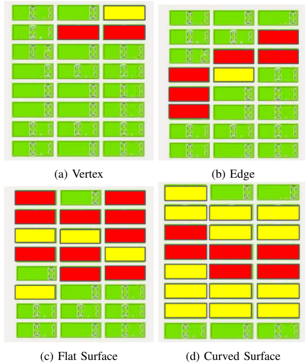
Fig. 2: Detection of different shape primitives on the fingers and palm of the Barrett Hand.
