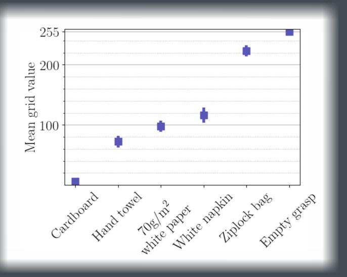
translucency and thickness. We have shown that a well-calibrated sensor can even detect a clear plastic ziplock bag.
